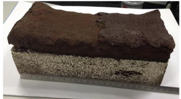
Figure 1: Brick of size 240mm x 120mm x 30 mm produced from custom 3D printing protocol at DLR's solar oven in Cologne. Support is made from a porous silica brick and JSC-2A is used as lunar simulant.
